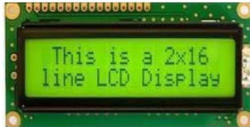
Gambar 6. LCD (*Liquid Crystal Display*)
